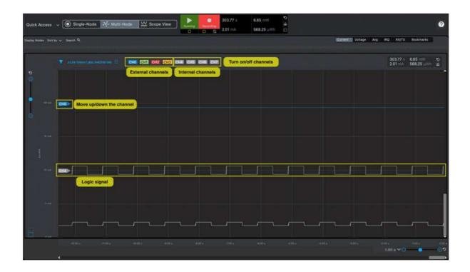
Freeze triggers can be set for the logic signals as for other features, as described in Freeze and Record Triggers. Click the Freeze trigger to open the configuration dialog, then select DigitalSignal, the target channel, and the condition.
